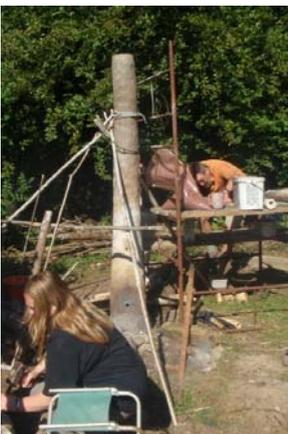
Two unusual furnaces were of note. One mini furnace, standing c50cm tall, produced no useable or even identifiable bloom. At no point did it seem to do what it was meant to do.
