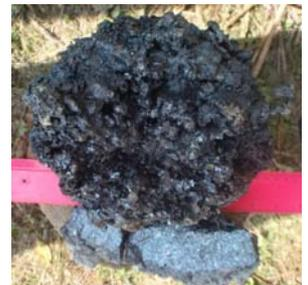
Gerry's furnace also made use of the electric pump for the air flow. A worthy bloom was produced but I detected no great air of rejoicing about its quality, possibly due to impurities within it but I cannot be sure.
