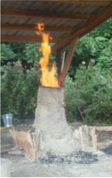
Gerry McDonnell supervised a furnace which roared with fire and the flames, and sparks were very evident throughout the process (others tended to create high temperature heat hazes and smoke). While not set into the ground, a bank of soil (held in place with planks) had been built up around this furnace. This may have held the heat in and also enabled the slag and bloom to be pulled out from the front of the base of the furnace at ground level instead of into a slag pit.
