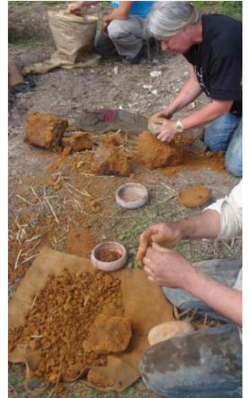
Iron ore of medium to poor quality was sourced mainly from one geographical location and supplied in large iron-bearing blocks of stone (just within carrying weight). These were pounded by hand using basic unfashioned handheld stones (the modern tool users used regular hammers to do the same job and the consistency was noticeably different as a result) on flat stones and log ends until the ore fragments were about pea sized or slightly larger.
