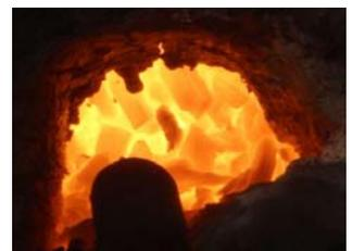
An electric air pump provided a noticeably more reliable air flow for all these furnaces. This air flow could be measured (air per litres). There was some debate about the merits of scientific measurement combined with a determination to produce a bloom vs. the authenticity of ancient methods.
