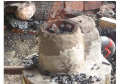
The bars were introduced vertically, one by one and they each sank into the charcoal as the base melted. The furnace was allowed to burn down and the remaining charcoal scooped out so that the button could be lifted out with tongs. On testing the metal, it was determined that it hadn't worked as well as they hoped and that nearly half the metal had been lost in the process, but it was an indication of how the process worked.
