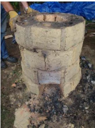
A particularly successful furnace was operated by an American team who had worked on Jamestown reconstructions. However, they used firebricks lined only internally by clay (which degraded between the bricks during the process). The furnace was built on the surface of the ground and these factors make it all very different to the archaeological evidence of sunken, stone-built medieval furnaces found on Iron-Age (Nidderdale) Project's site.
