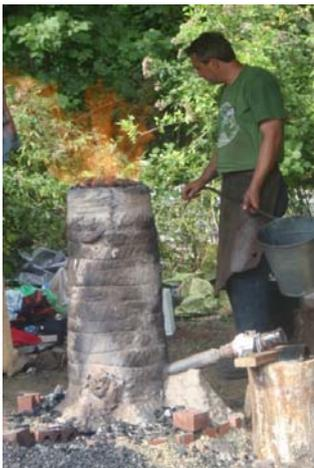
A second successful furnace made by the Americans was thinner in shape and both lined and coated by clay. Its base seemed to have been set into the ground and insulated by brick.
